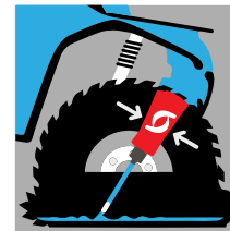
STEP 2 - INSTALL LIQUID TIREJECT®
